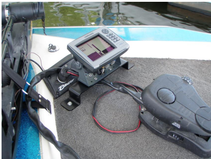
Blazer Bow Mount Bracket - On Deck Installation
